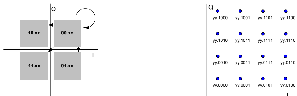
Fig. 74 Symbol mapping D64 QAM / DVB-C
